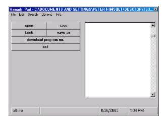
The TS312 terminal software is checking eery 5 seconds for the serial communication with the position controller. The status of the left window will change to "online" if the serial communication works properly. The next window to the right will then show the "max. program number" to be downloaded as entered in parameter All/P60 of the positioning controller (see controller manual)
