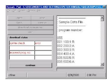
Note: The PS312P Position controller must be in "Single Positioning Mode" to accept program download. Downloading in Program Mode or Manual Mode is not allowed
